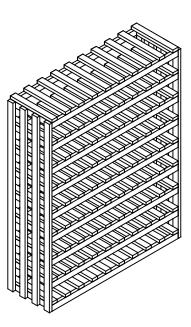
5. Middle Stack and Top Stack rack can be place directly on top.
